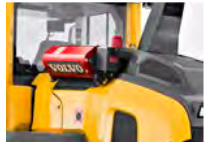
Fire suppression system
