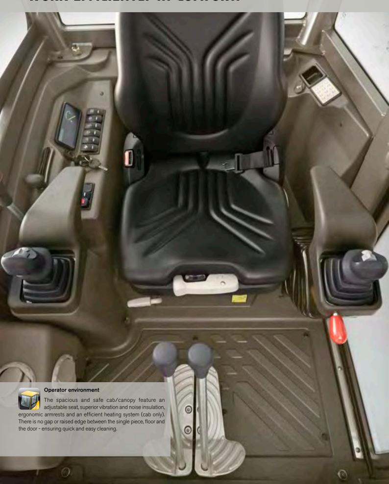
Step inside the spacious ECR25D and experience the benefits of the comfortable and intuitive Volvo operator environment. The modern styling delivers superior all-around visibility from large expanses of glass as well as innovative, ergonomic features including ideally placed controls and heavy a large floor - with no auxiliary pedals - for increased foot space.
