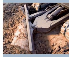
Hydraulic angle blade rotates to save time.
