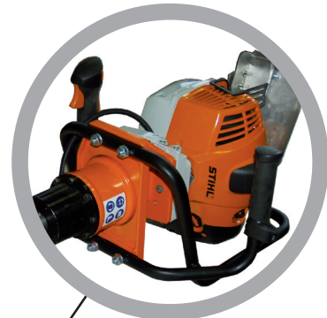
ergonomic handles for one-man operation
